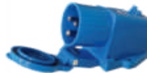
CEE surface-mounted power socket Ideal for concealed installation in the engine compartment (e.g. on T5) with cover 3-pole 230 V / 16 A. 82008 13,90
